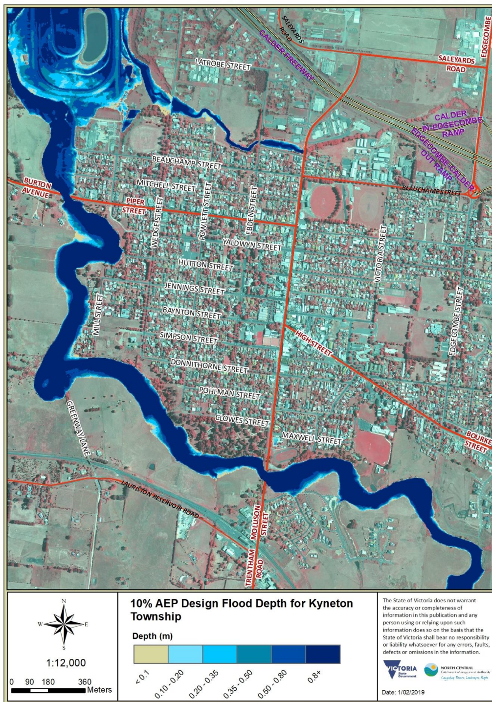
Figure 7-4 10% AEP design flood depth for Kyneton Township
