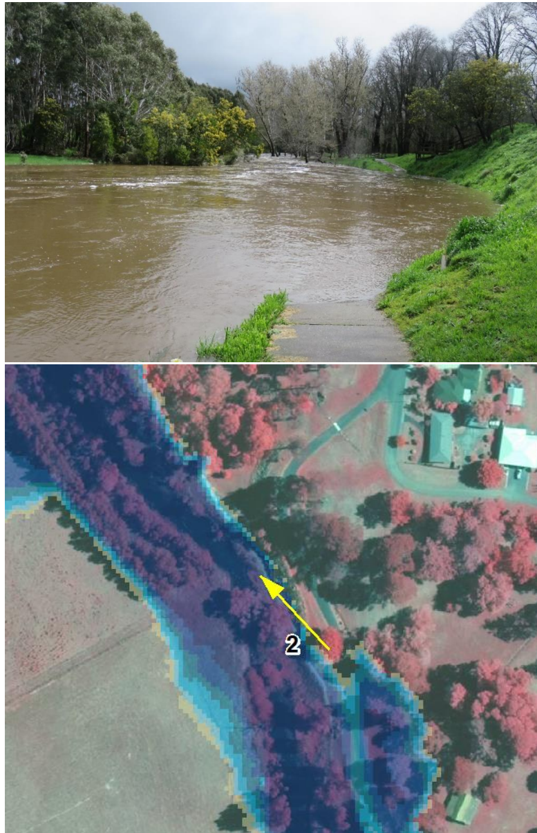
Figure 4-25 Comparison of modelled flood extent to photo taken during the September 2016 event looking downstream on the Campaspe River from the Kyneton Botanic Gardens
