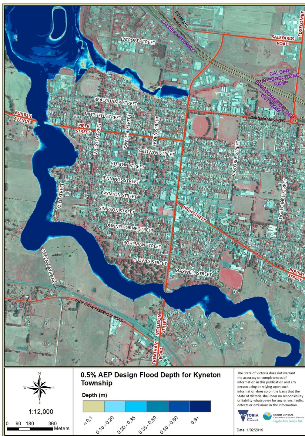
Figure 7-12 0.5% AEP design flood depth for Kyneton Township
