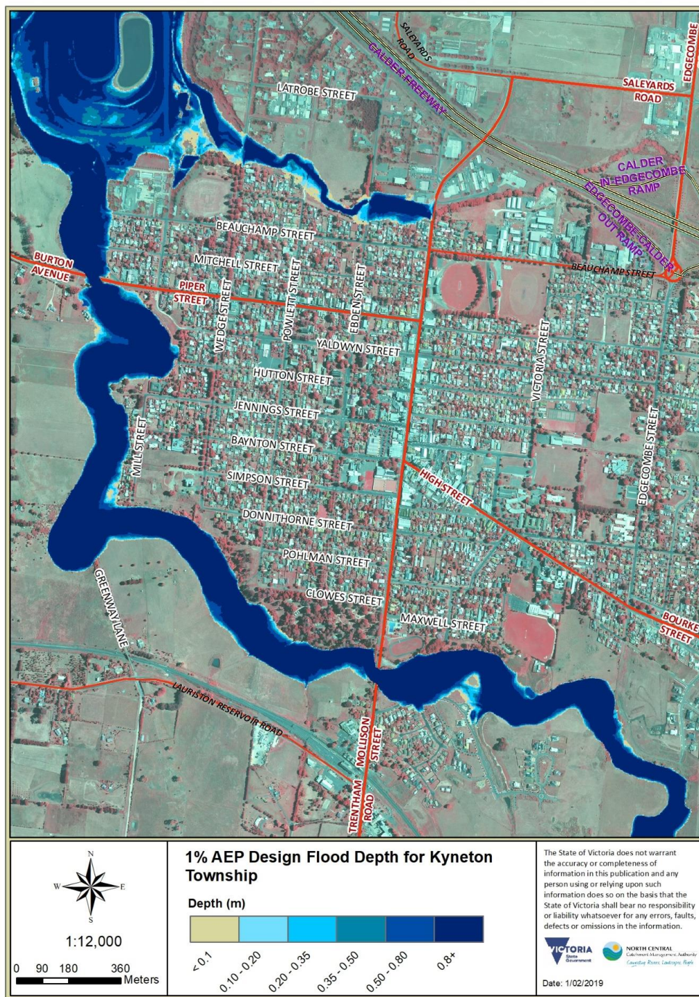
Figure 7-10 1% AEP design flood depth for Kyneton Township
