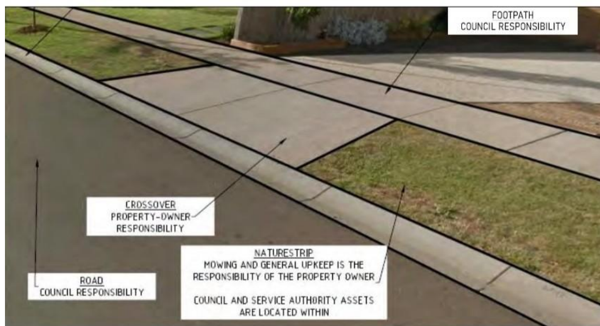
TYPICAL VEHICLE CROSSING DIAGRAM
