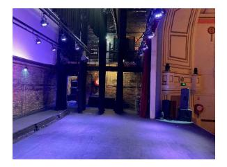
Fly Galleries protrude **1200mm** at a height of **2550mm** from OP and PS Walls.
