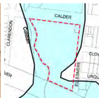
Figure 7. LSIO - Land Subject to Inundation - identifies land in a flood storage or flood fringe area affected by the 1 in 100 year flood. Development needs to maintain or improve river and wetland health, waterway protection and flood plain health.
