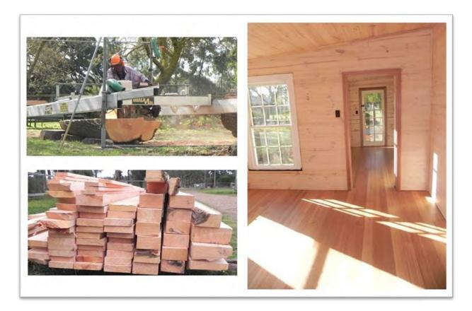
Figure: Portable saw mills are a game changer for small scale boutique farm forestry. Timber can be cut and dried on farm and used or sold for high value uses such as house floor boards and benches. Photos:
