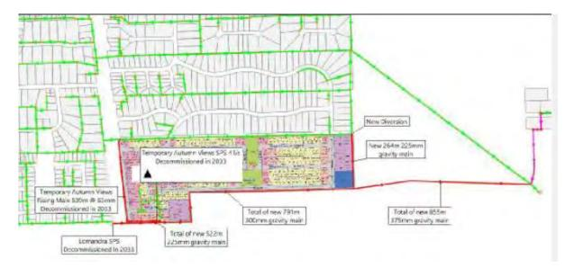
GWW has advised that generally land to the south of this is too low to be controlled by the existing sewer. A dedicated sewerage pump station and rising main back to the RWP would be required to service growth to the south.
