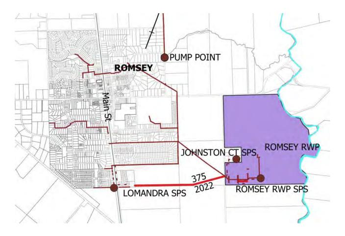
The majority of the existing town is sewered via gravity to the RWP for treatment. The low density residential area is not sewered. The Pump Point shown to the north east of town is part of the system that conveys sewage from Lancefield to the RWP for treatment.
