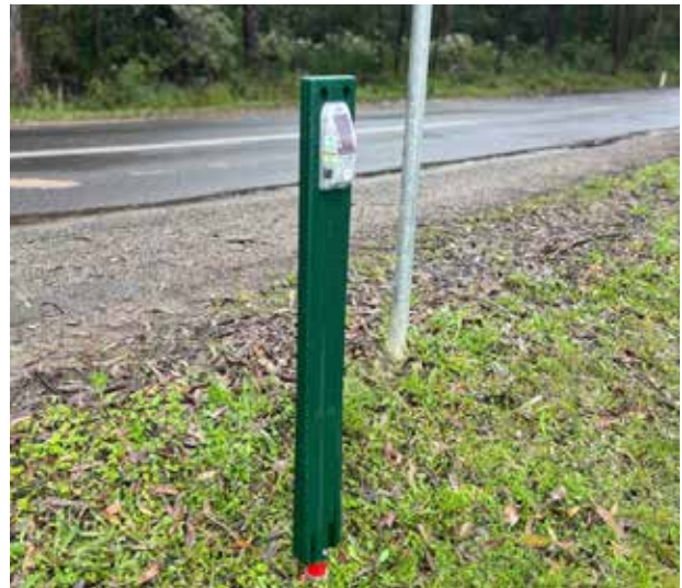
Virtual fencing emits sound and flashing lights to alert animals to oncoming vehicles.
