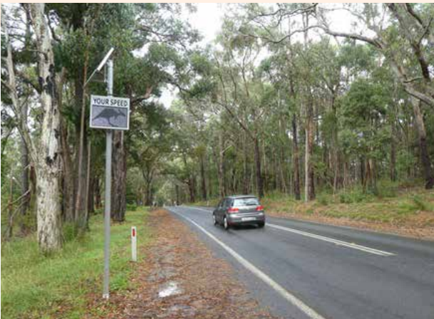
Solar-powered variable message sign. Photo sourced from Mirage News
