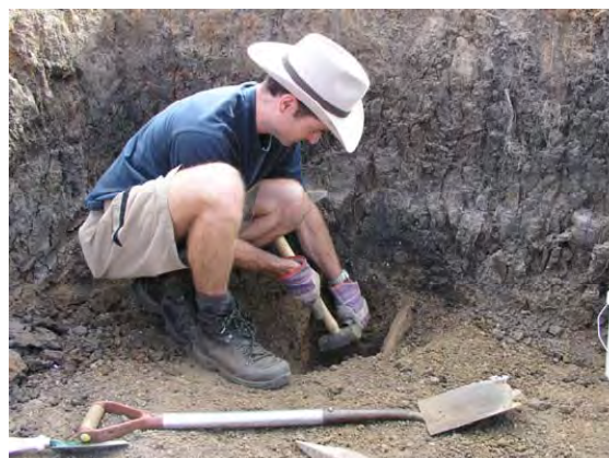
Matt Cupper hammers in tubes to collect sediments for luminescence dating
