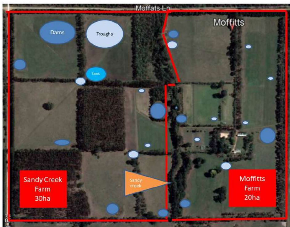
Figure: Sandy Creek farm has livestock water supplied from dams, Sandy Creek and reticulated water pumped to a header tank and redistributed by gravity flow to trough place at the centre of paddock “wagon wheels”.
