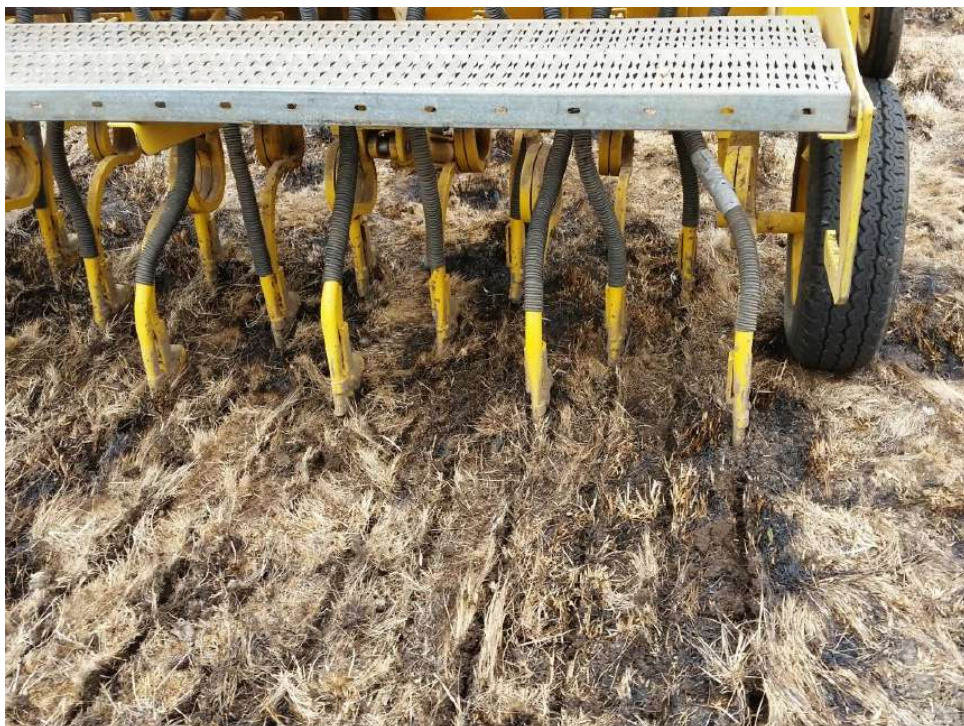
Figure: Direct drilling pasture seed minimises soil disturbance ensuring soil organic carbon is protected , soil food web habitat is maintained and tractor emissions are minimal while introducing more productive species.
