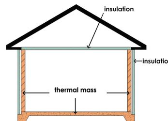
Figure 6.2: Thermal mass within the insulated envelope
