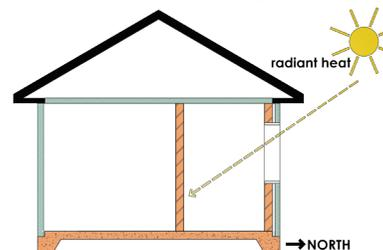
Figure 6.3: Locate thermal mass in north facing rooms.
