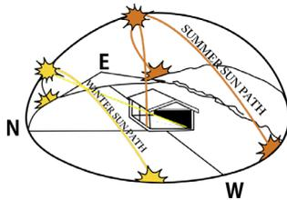
Figure 1.2 Altitude and Azimuth
