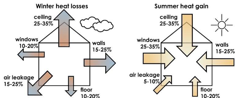
Typical heat losses and gains without insulation in a temperate climate
