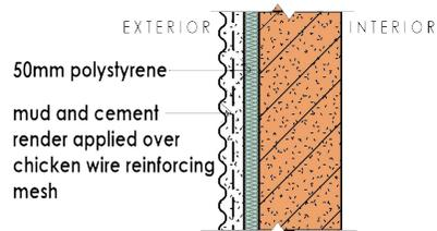
Figure 6.5: Insulation fixed to the outside of the mud brick
