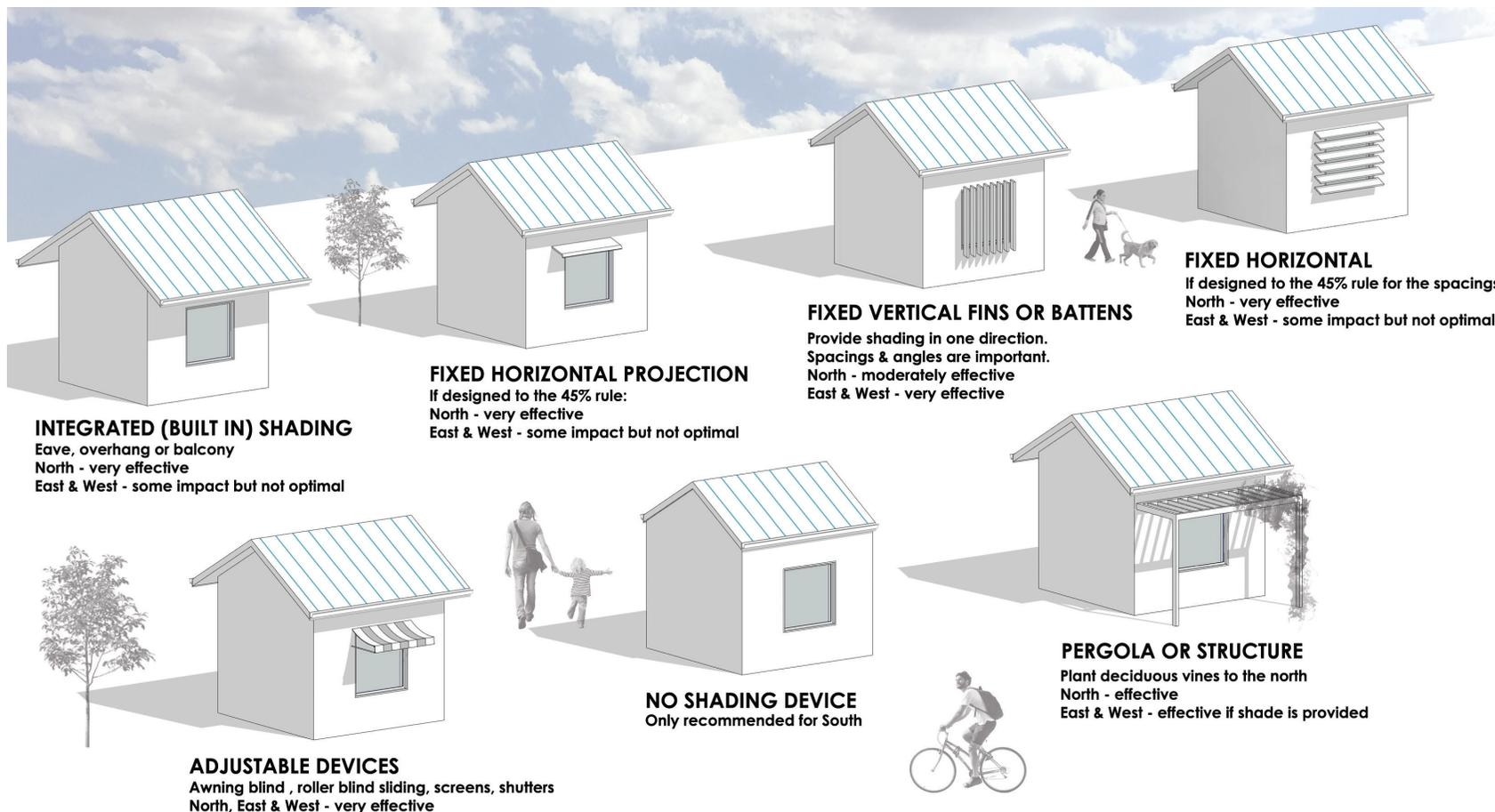
**INTEGRATED (BUILT IN) SHADING**
