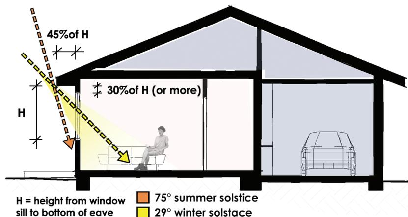
Using this 45% rule, eave overhangs should be:
