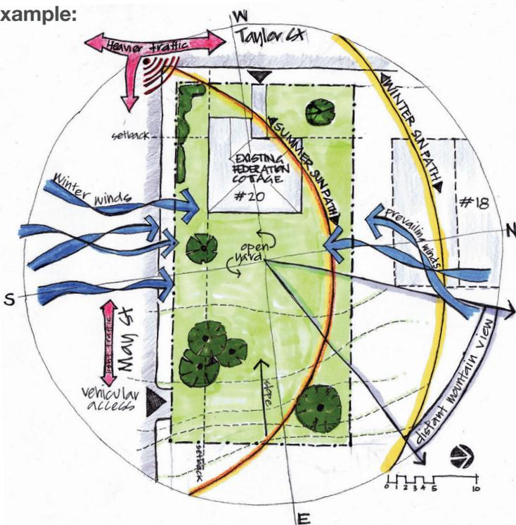
Figure 1.5 Site analysis: study for proposed addition to existing cottage
