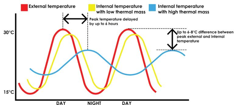
Figure 6.1: Stabilising effect of thermal mass on internal building temperatures.
