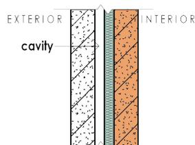
Figure 6.6: Insulation fixed to the outer side of the inner mud brick leaf
